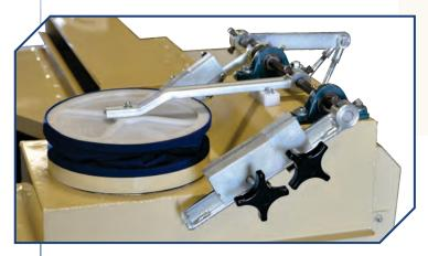
**Automatic Discharge System** senses product depth and adjusts the discharge gate for fluctuations in product flow. This consistent bed depth eliminates constant readjustment.
