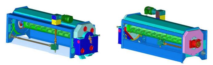
The Modular Drive System uses a motor mounted right angle reducer which connects to a PTO shaft. The PTO shaft then connects to a 3 way transfer box which directs power to the end of the cylinder.
