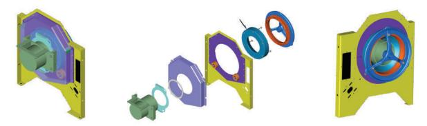
Patent Pending Carter Day Urethane Seal offers a unique shaft sealing system stopping grain from flowing back to the inlet which stops leakage. This seal has been critical working with canola and small seed applications.
