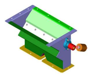
The optional **Weighted Gate Feeder** for the Modular Uniflow and No. 3SI for inlet feed control. The weighted gate offers a more controlled length separation and restricts over filling of the cylinder which may cause inlet leaking.
