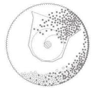
arated depends on the number of pockets coming in contact with the product and lifting edge. The optional adjustable retarder system found on the Modular Uniflow and No. 3SI may also be used to control the amount of product maintained in the cylinder. The adjustable retarder can be positioned out of the product flow when it is not required.
