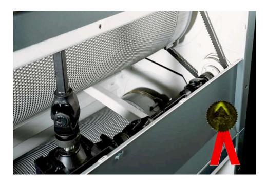
angle reducer which connects to a PTO shaft. The PTO shaft then connects to a 3 way transfer box which directs power to the end of the cylinder.
